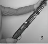
Cycle the bolt manually several times and make sure that the bolt is going forward to the fully locked position. Refer to the photographs above to ensure that you are assembling your shotgun correctly.
