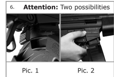
**Remove the magazine:** **1.** Standard Remove by pushing the magazine release lever. **2.** When the magazine release lever is in opposition to the nose of the loading disc (pic. 1), push the magazine release button on the right side (pic. 2)
