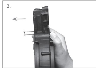
2. Remove the screws from the magazine head.
