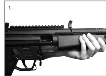
**Attention:** The ejection port must be always opened and locked, when you insert the magazine.
