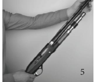
Cycle the bolt manually several times and make sure that the bolt is going forward to the fully locked position. Refer to the photographs above to ensure that you are assembling your shotgun correctly.
